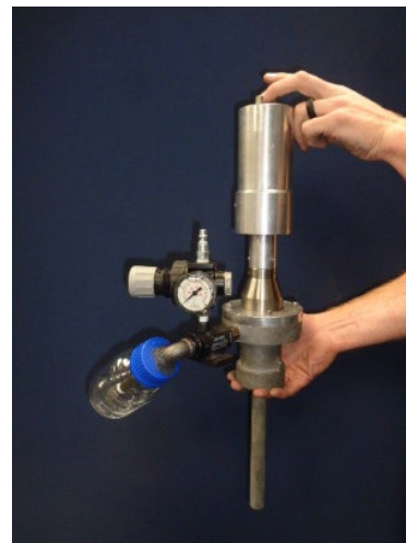
Figure 1. Modified ultrasonic head unit.
