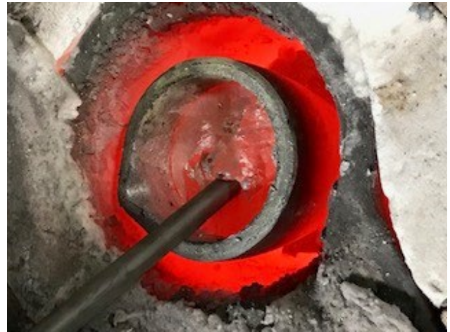
Figure 4. Fluidized particle delivery in molten metal.
